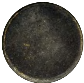
Before - Typical fouled diffuser
